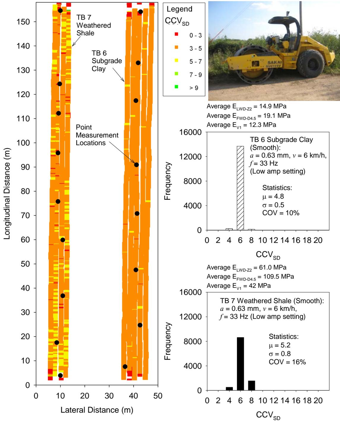
Figure 52.  $CCV_{SD}$  map and histogram plots for TBs 6 and 7 (low amplitude setting)
