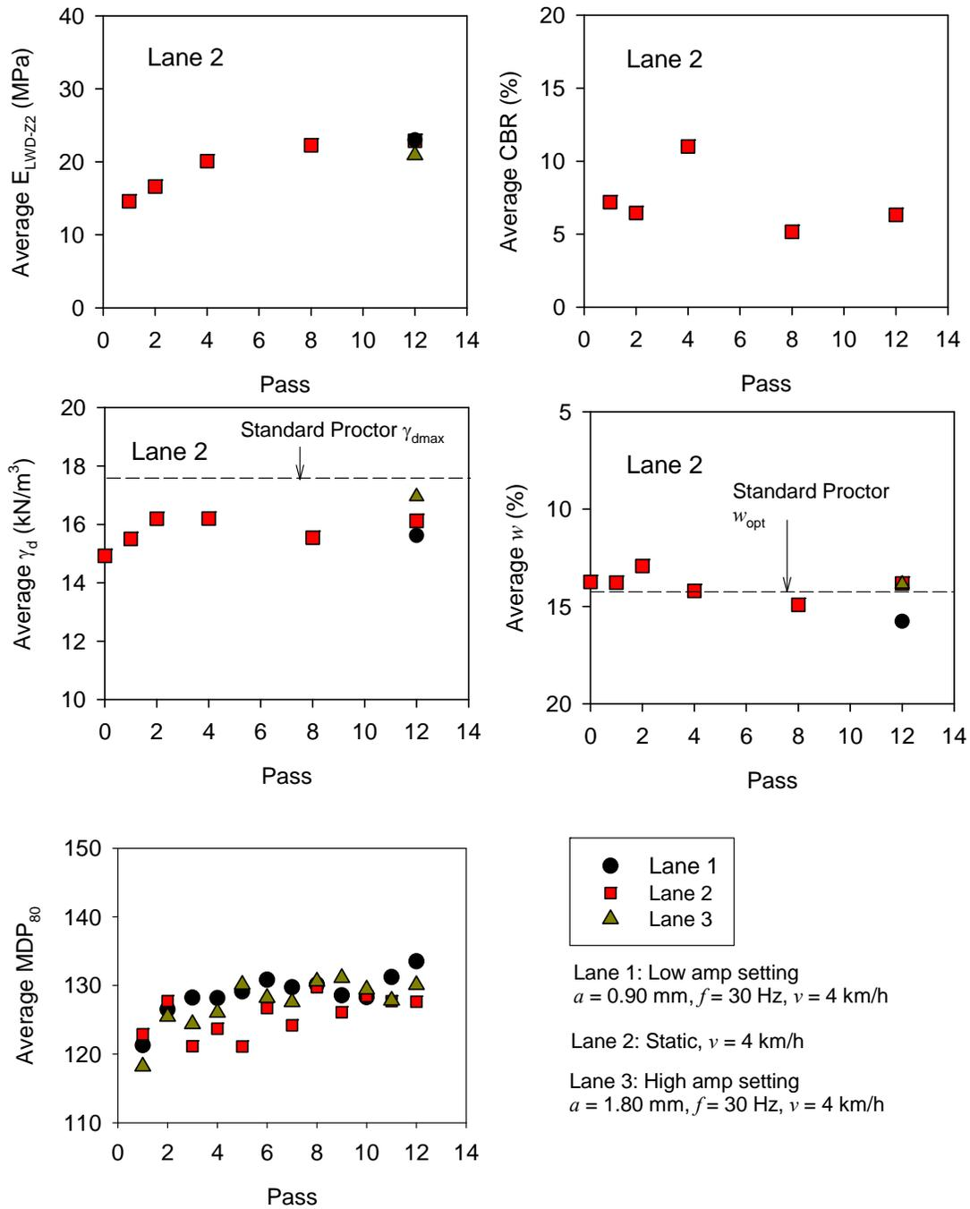
**Figure 22. Comparison between average in-situ point measurement and average  $MDP_{80}$  per pass compaction growth on TB2 subgrade clay material**
