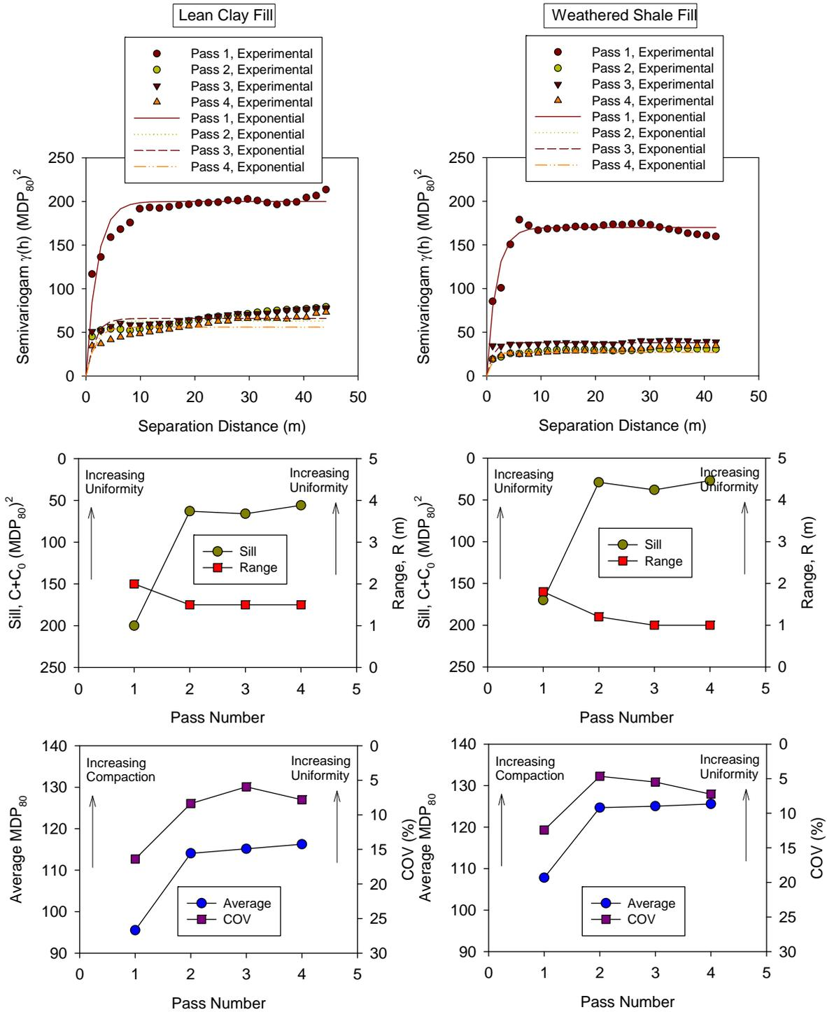
**Figure 44. Change in semivariograms, spatial statistics, and univariate statistics of  $MDP_{80}$  with pass on TB3 – lift 3 lean clay and weathered shale fill materials**
