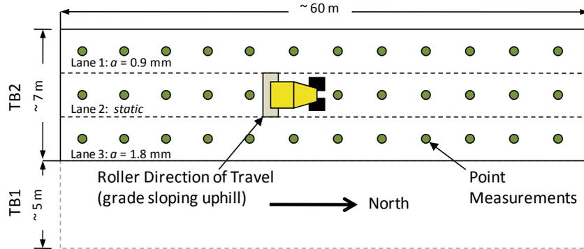
**Figure 16. Experimental testing setup on TB2 (TB1 shown for reference)**
