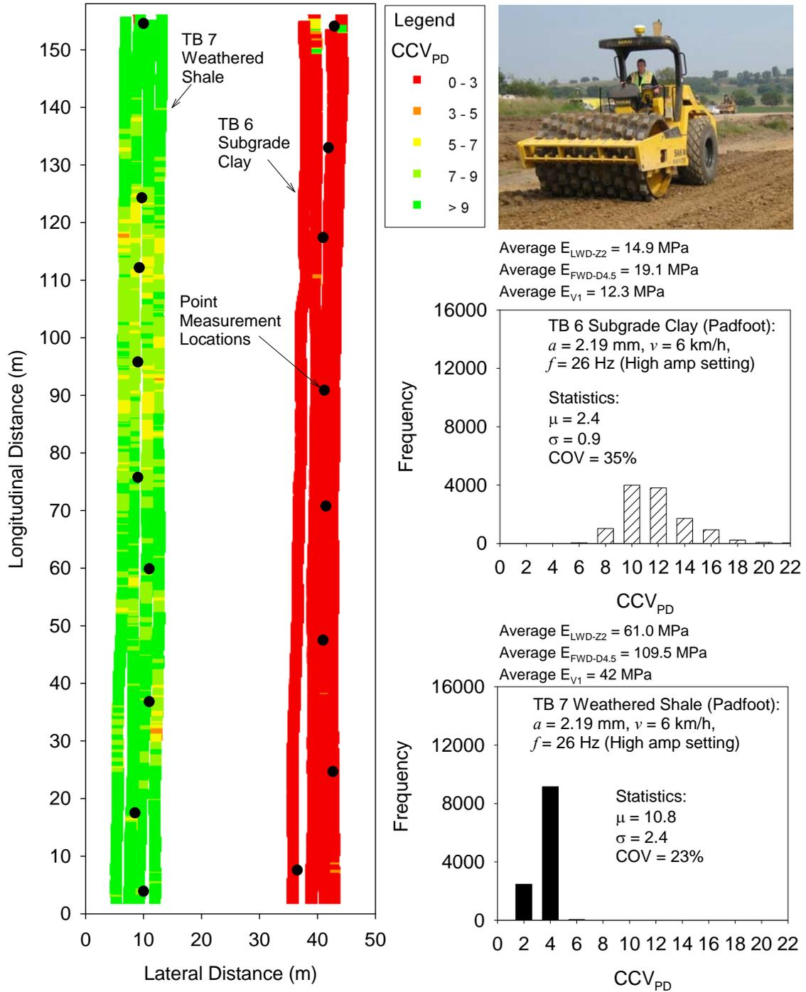
Figure 51.  $CCV_{PD}$  map and histogram plots for TBs 6 and 7 (high amplitude setting)
