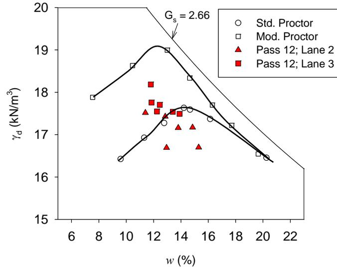
**Figure 30. Comparison between laboratory  $w$ - $\gamma_d$  relationship and in-situ  $w$ - $\gamma_d$  point measurements after final pass on lanes 2 and 3 – TB 4 subgrade clay (USCS: CL)**
