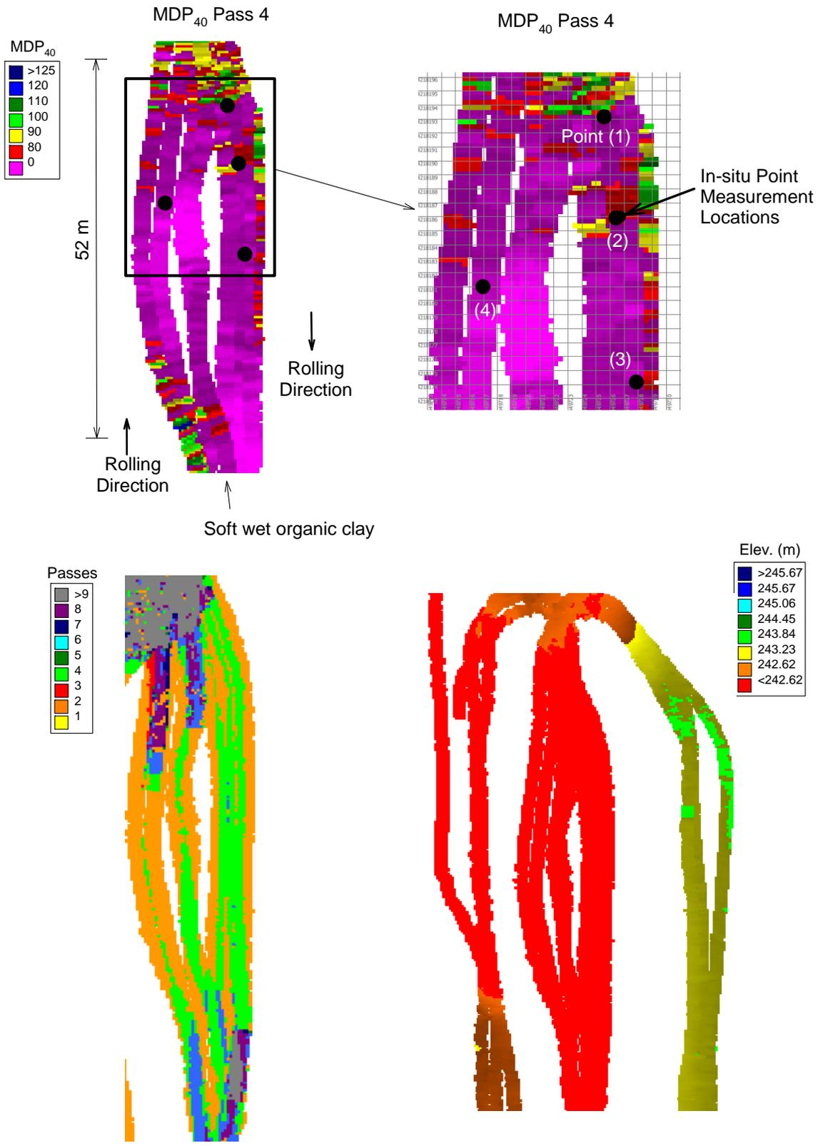
Figure 46. MDP<sub>40</sub> (static mode,  $v = 4$  km/h) measurements on pass 4, elevation, and pass coverage information – TB5 wet organic clay
