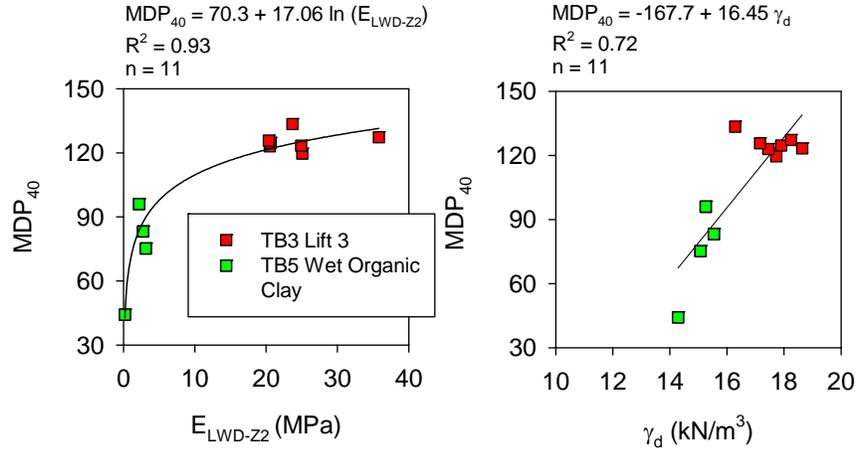
**Figure 64. Regression relationships between  $MDP_{40}$  and in-situ point measurement values – TB3 lift 3 ( $a = 0.90$  mm,  $f = 33$  Hz) and TB5 (static)**
