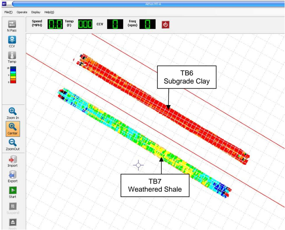
**Figure 49. AithonMT display of  $CCV_{SD}$  map ( $a = 1.48 \text{ mm}$ ,  $f = 26 \text{ Hz}$ )**
