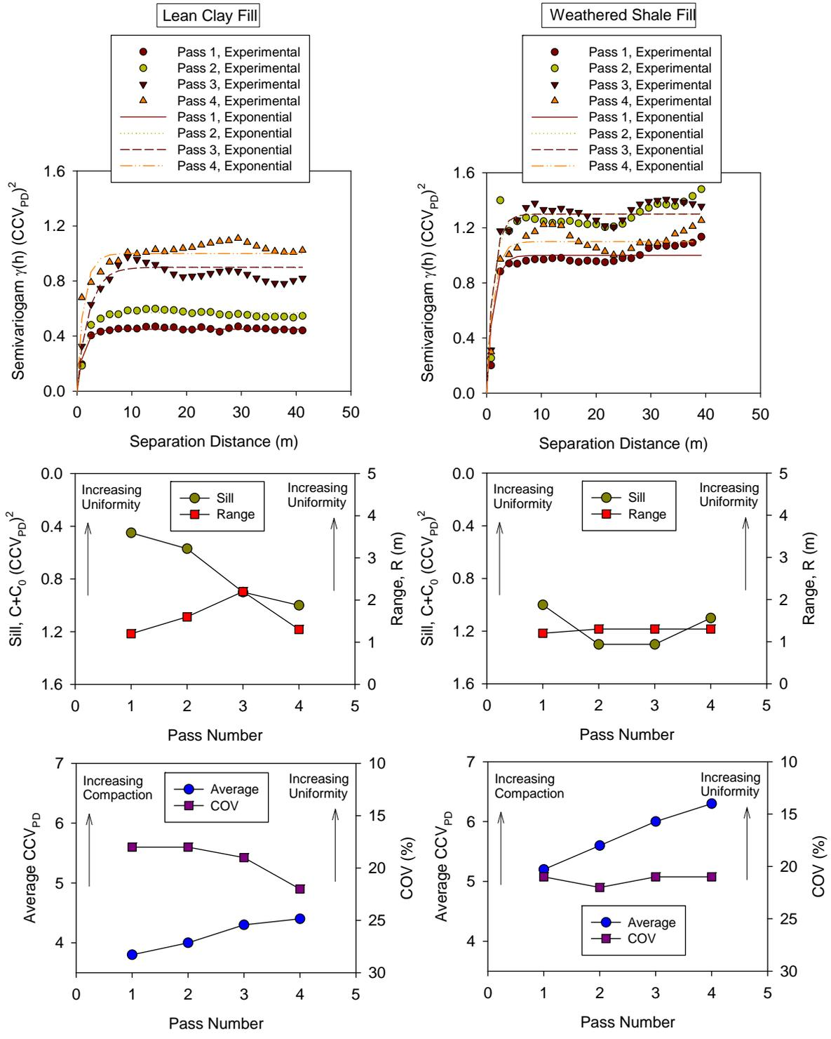
**Figure 45. Change in semivariograms, spatial statistics, and univariate statistics of CCV<sub>PD</sub> with pass on TB3 – lift 6 lean clay and weathered shale fill materials**
