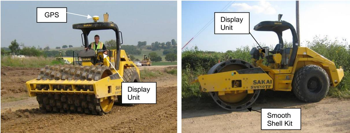
**Figure 2. Sakai SV610 roller with padfoot and smooth drum setup used on the project**
