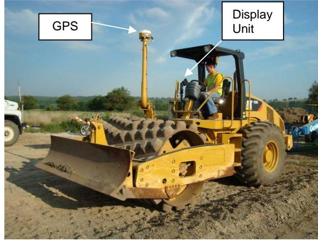
**Figure 3. Caterpillar CS56 padfoot roller used on the project**
