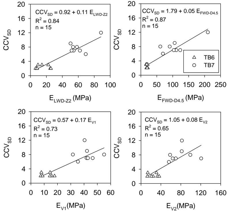
**Figure 58. Regression relationships between  $CCV_{SD}$  and in-situ point measurement values from TBs 6 and 7 ( $a = 1.48$  mm,  $f = 26$  Hz)**
