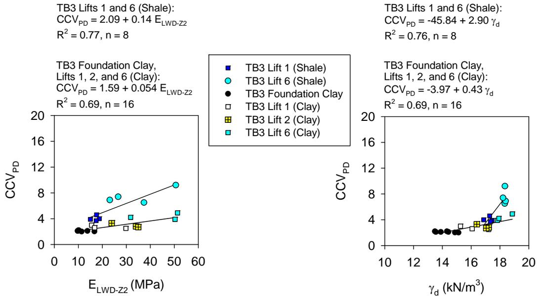
**Figure 57. Regression relationships between  $CCV_{PD}$  and in-situ point measurement values from TB3 production area ( $a = 2.19$  mm,  $f = 26$  Hz)**
