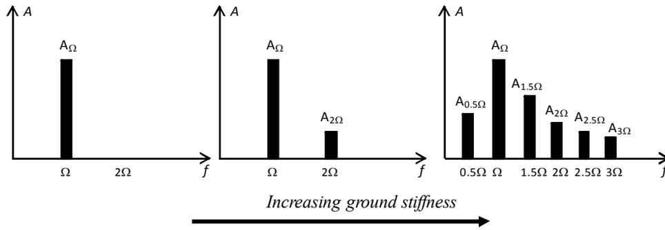
**Figure 1. Changes in amplitude spectrum with increasing ground stiffness (modified from Sakai Manual)**
