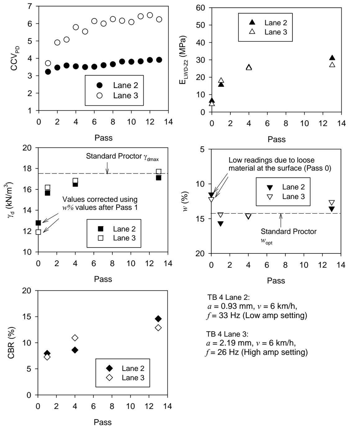
**Figure 29. Comparison between CCV and in-situ point measurement compaction growth (average values per pass) with increasing roller passes – TB 4 lanes 2 and 3 subgrade clay (USCS: CL)**
