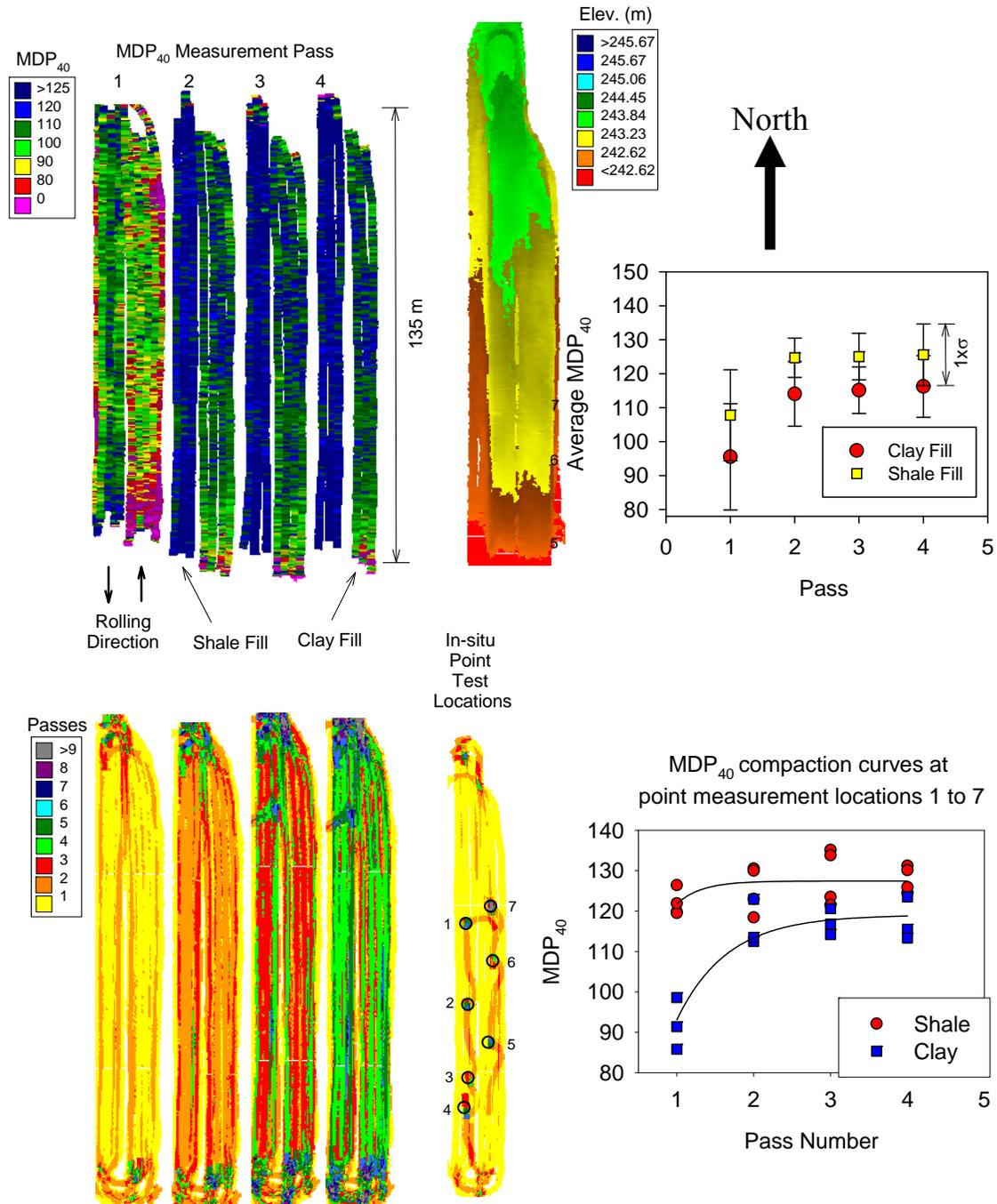
**Figure 39. MDP<sub>40</sub>, elevation, pass coverage, average MDP<sub>40</sub> ( $a = 0.90$  mm,  $f = 33$  Hz,  $v = 4$  km/h) per pass, and MDP<sub>40</sub> at select point locations on TB3 lift 3 clay fill and shale fill material**
