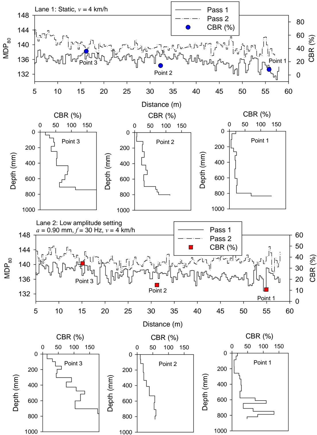
**Figure 12. Comparison between  $MDP_{80}$  and DCP-CBR point measurements –TB1 subgrade clay material (note: passes 1 and 2 with opposite machine direction of travel)**
