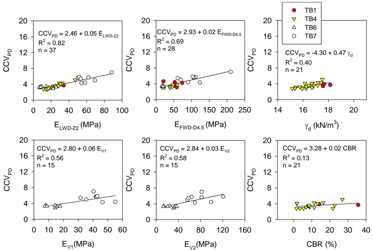
**Figure 56. Regression relationships between  $CCV_{PD}$  and in-situ point measurement values from TBs 1, 2, and 4 calibration test strips, and TBs 6 and 7 ( $a = 0.93$  mm,  $f = 33$  Hz)**
