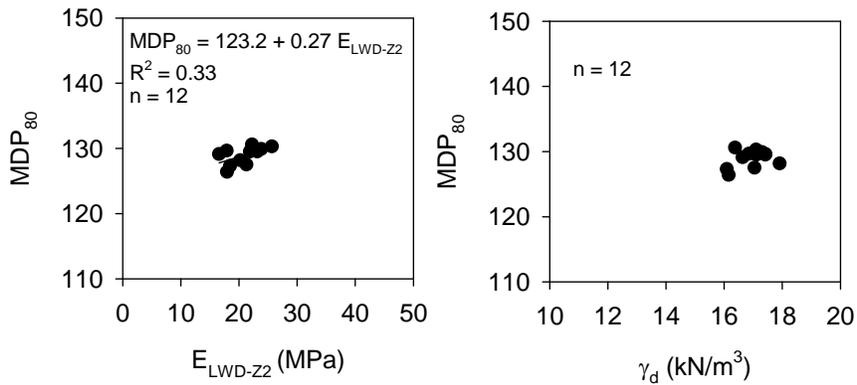
**Figure 61. Regression relationships between  $MDP_{80}$  ( $a = 1.80$  mm,  $f = 33$  Hz, driving uphill) and in-situ point measurement values – TB2 subgrade clay**
