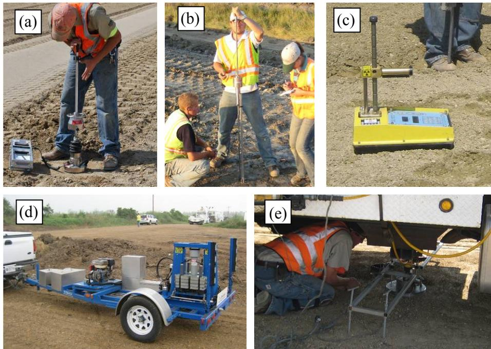
**Figure 4. In-situ testing methods used on the project: (a) 200-mm plate diameter Zorn LWD, (b) dynamic cone penetrometer, (c) nuclear moisture-density gauge, (d) KSDOT 450-mm plate diameter Dynatest FWD, and (e) 300-mm plate diameter static PLT**
