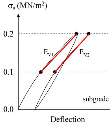
**Figure 5.  $E_{V1}$  and  $E_{V2}$  determination procedure from static PLT for subgrade materials**
