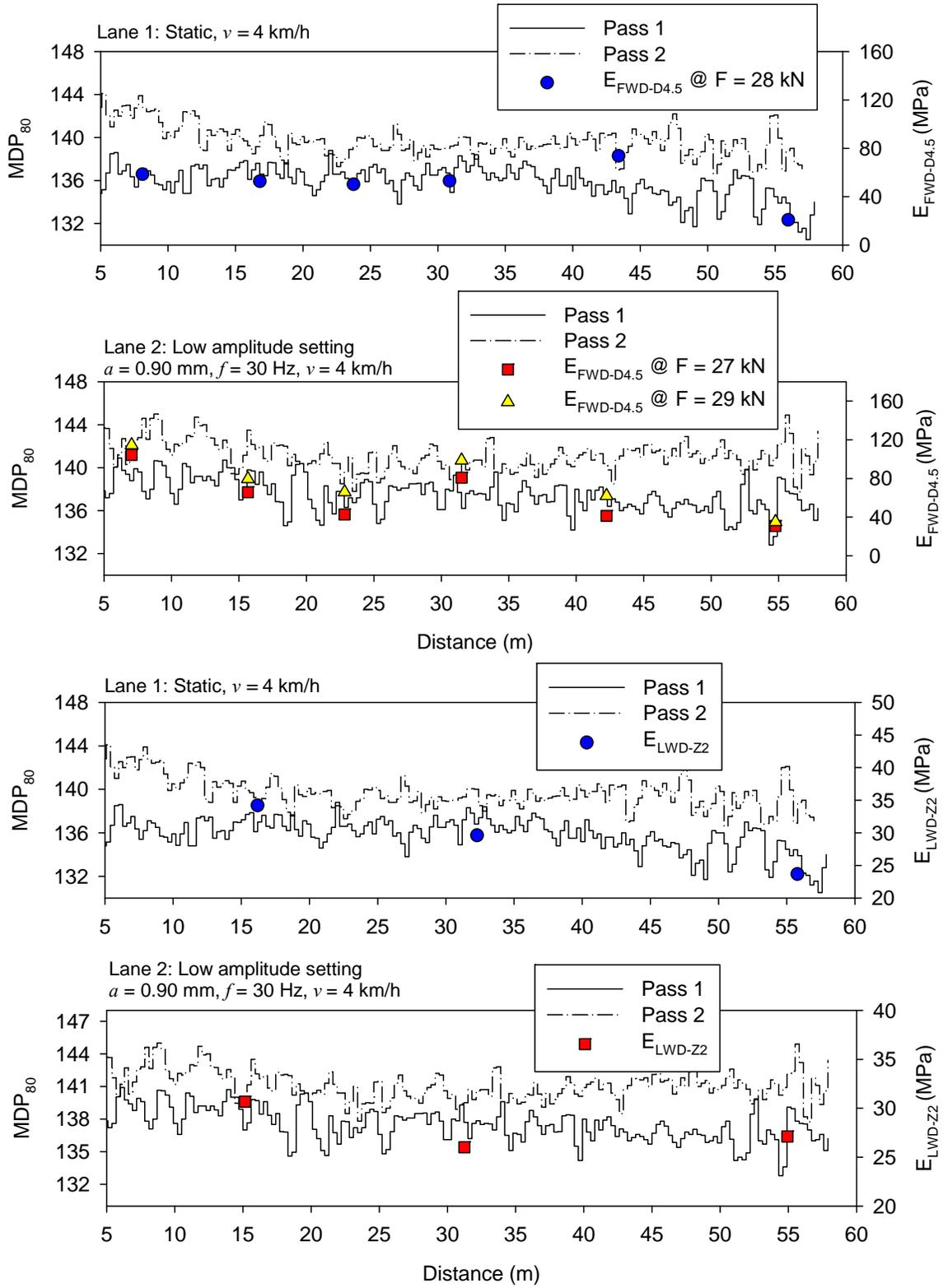
**Figure 10. Comparison between MDP<sub>80</sub> and E<sub>LWD-Z2</sub> (top) and E<sub>FWD-D4.5</sub> (bottom) point measurements – TB1 subgrade clay material (note: passes 1 and 2 with opposite machine direction of travel)**
