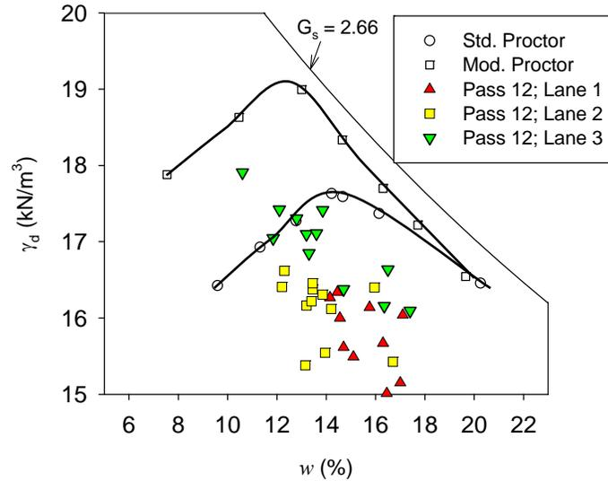
**Figure 23. Comparison between laboratory Proctor curves and in-situ moisture-dry unit weight point measurements after pass 12 on TB2 subgrade clay material**
