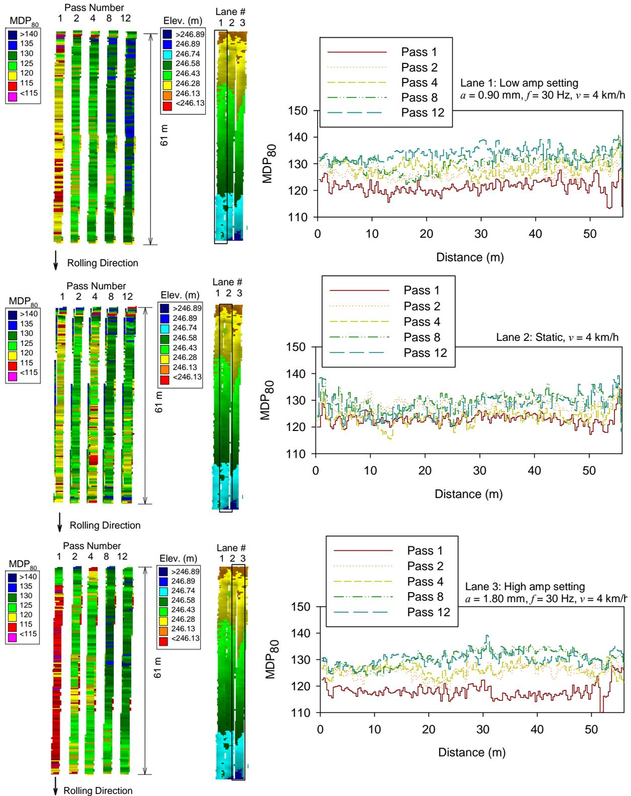
Figure 18. MDP<sub>80</sub> measurements for multiple passes on TB2 subgrade clay material lanes 1, 2, and 3
