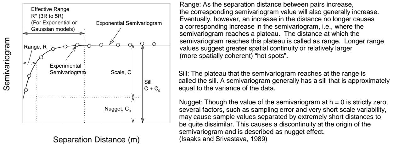
**Figure 43. Description of a typical experimental and exponential semivariogram and its parameters**
