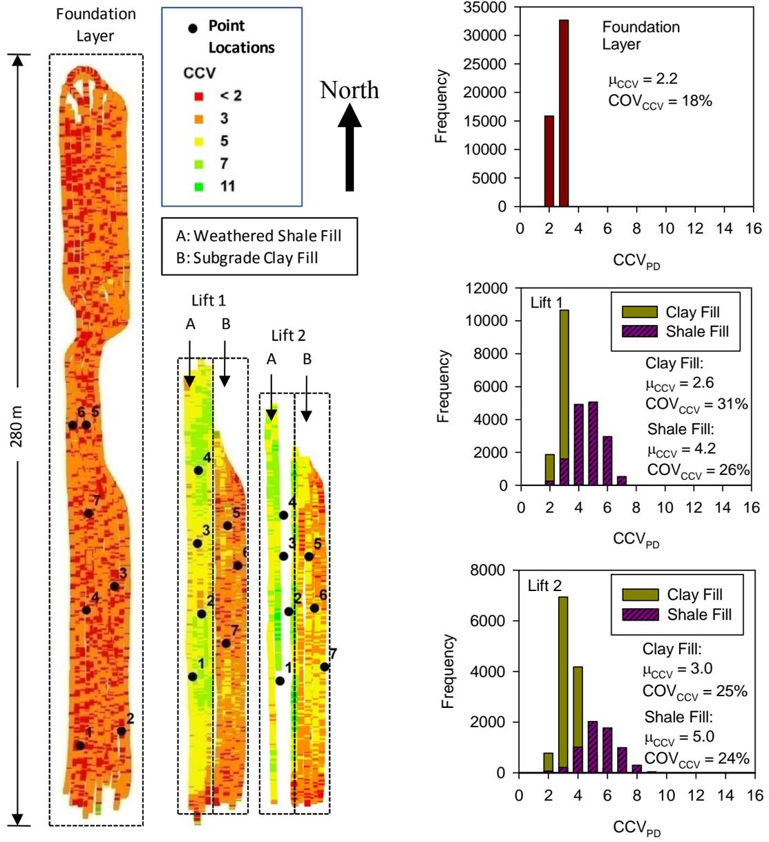
Figure 40.  $CCV_{PD}$  maps on foundation layer and lifts 1 to 2 ( $a = 0.93$  mm,  $f = 33$  Hz, and  $v = 4$  km/h)
