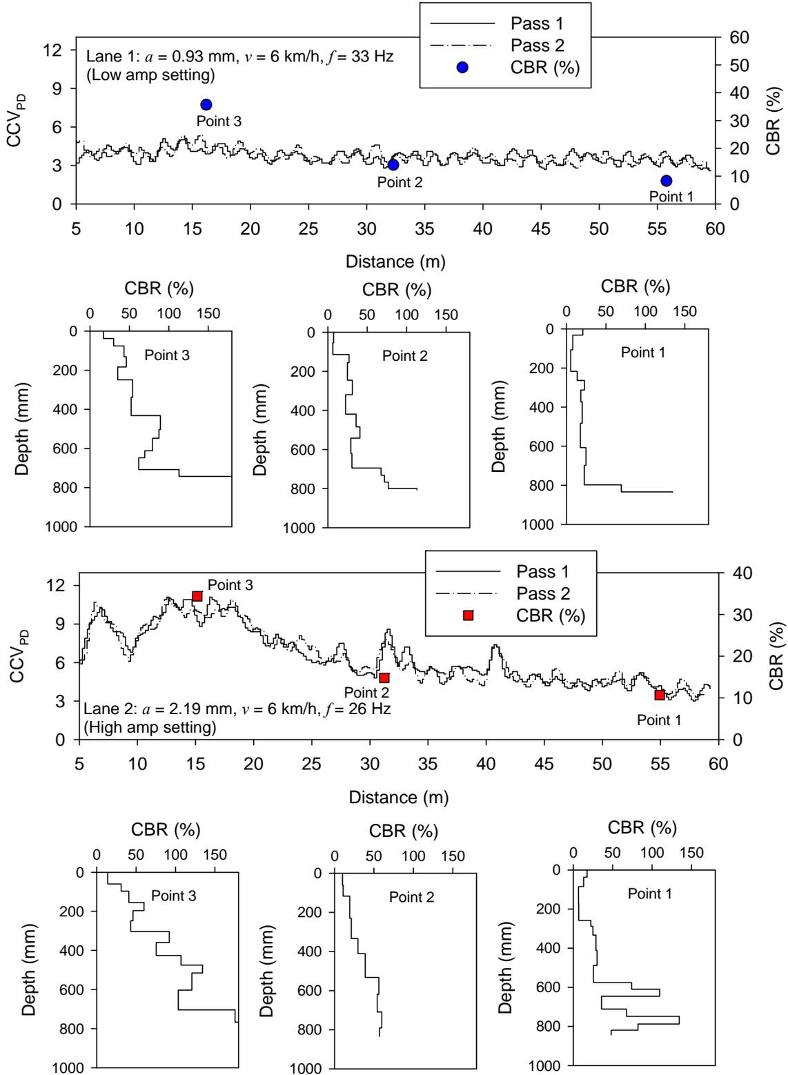
**Figure 15. Comparison between  $CCV_{PD}$  and DCP-CBR point measurements –TB1 subgrade clay material (note: passes 1 and 2 with opposite machine direction of travel)**
