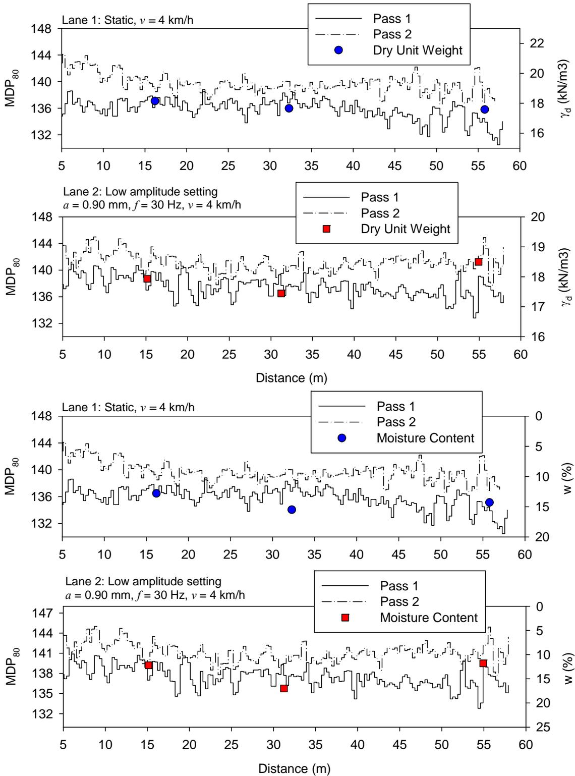
**Figure 11. Comparison between MDP<sub>80</sub> and nuclear moisture-density gauge point measurements – TB1 subgrade clay material (note: passes 1 and 2 with opposite machine direction of travel)**
