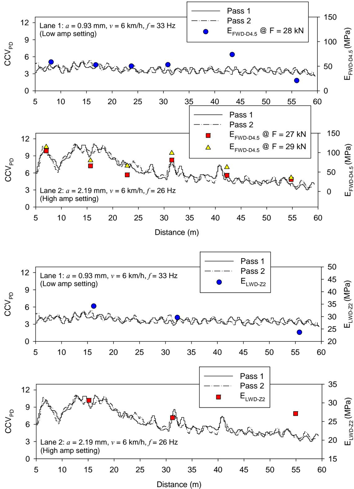
**Figure 13. Comparison between CCV<sub>PD</sub> and in-situ E<sub>FWD-D4.5</sub> and E<sub>LWD-Z2</sub> point measurements – TB1 subgrade clay material**
