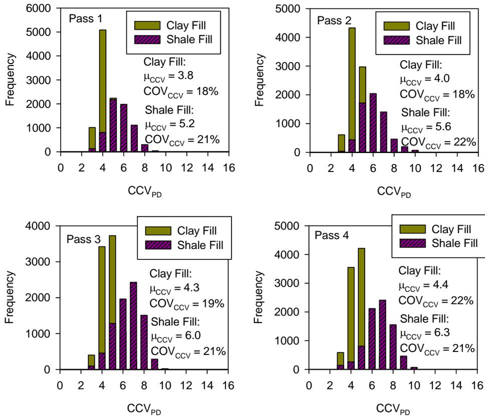
**Figure 42. Histogram plots of  $CCV_{PD}$  measurement values on lift 6 clay and weathered shale fill materials for passes 1 to 4**
