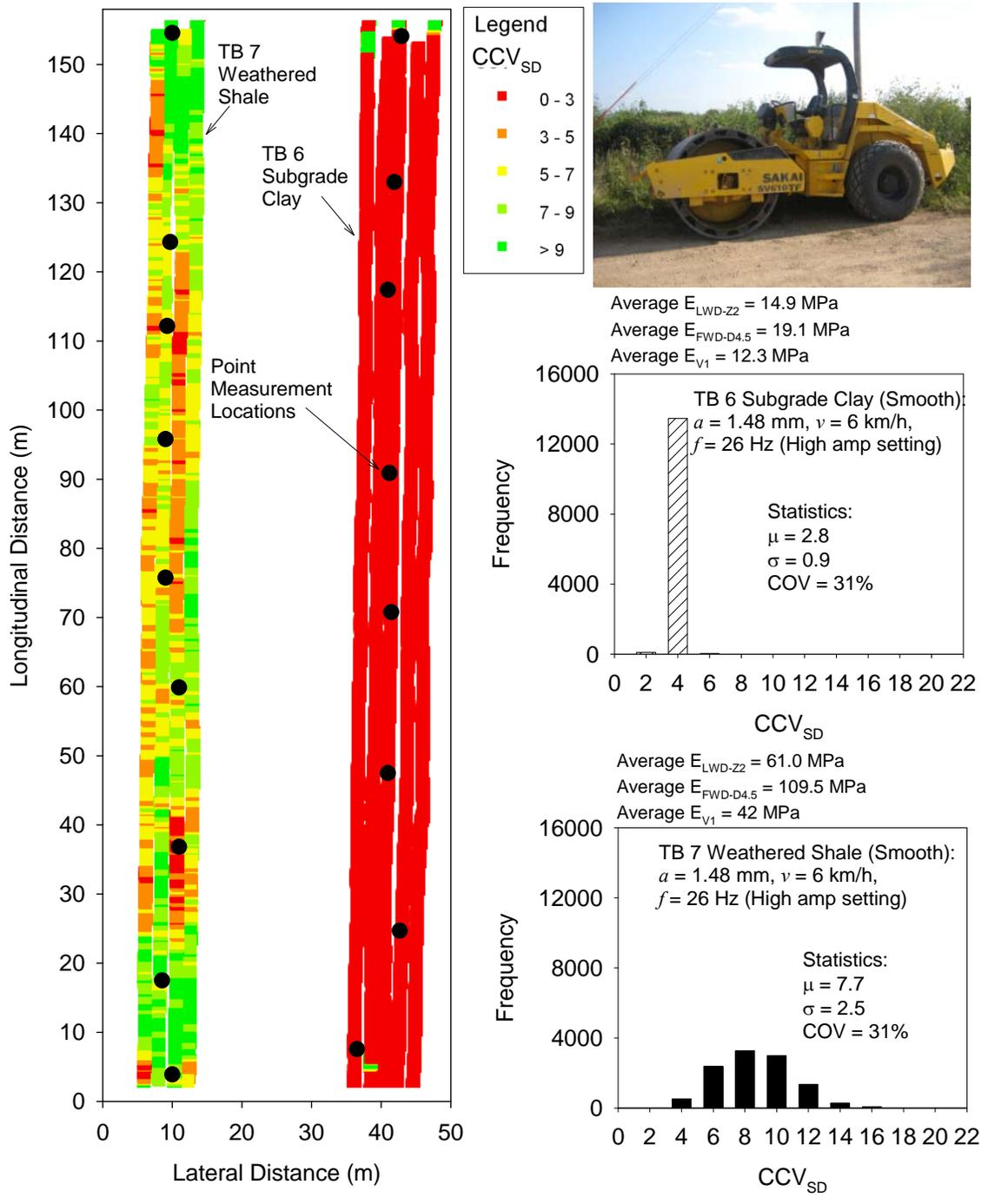
**Figure 53.  $CCV_{SD}$  map and histogram plots for TBs 6 and 7 (high amplitude setting)**
