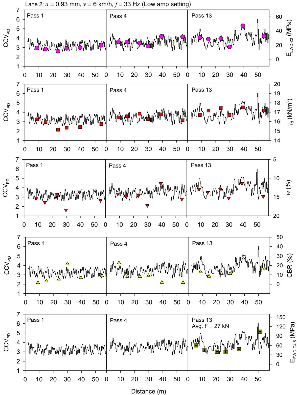
**Figure 27. Comparison between CCV and in-situ point measurements – TB4 lane 2 subgrade clay material (USCS: CL)**
