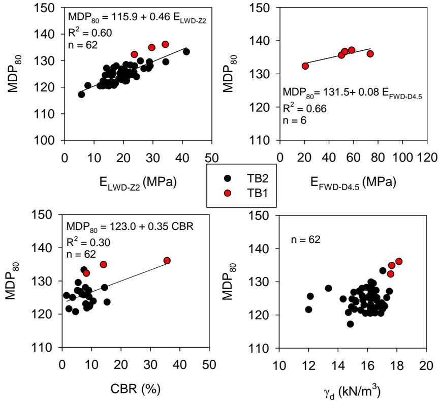
**Figure 60. Regression relationships between  $MDP_{80}$  (static – driving uphill) and in-situ point measurement values – TBs 1 and 2 subgrade clay**
