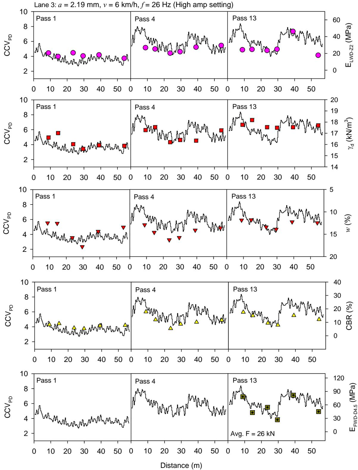
**Figure 28. Comparison between CCV and in-situ point measurements – TB4 lane 3 subgrade clay material (USCS: CL)**
