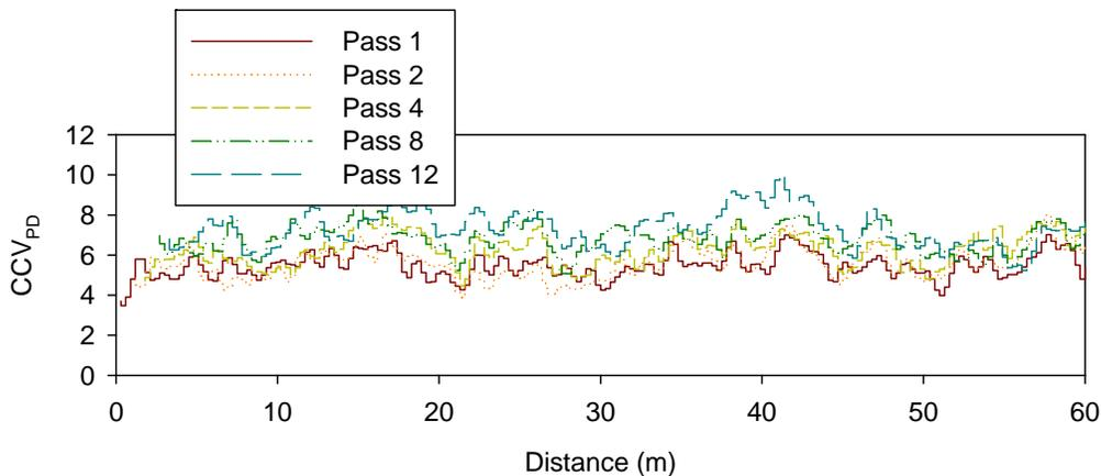
**Figure 31.  $CCV_{PD}$  measurements from multiple passes on TB3 lift 4 weathered shale fill material ( $a = 2.19$  mm,  $f = 26$  Hz,  $v = 6$  km/h)**
