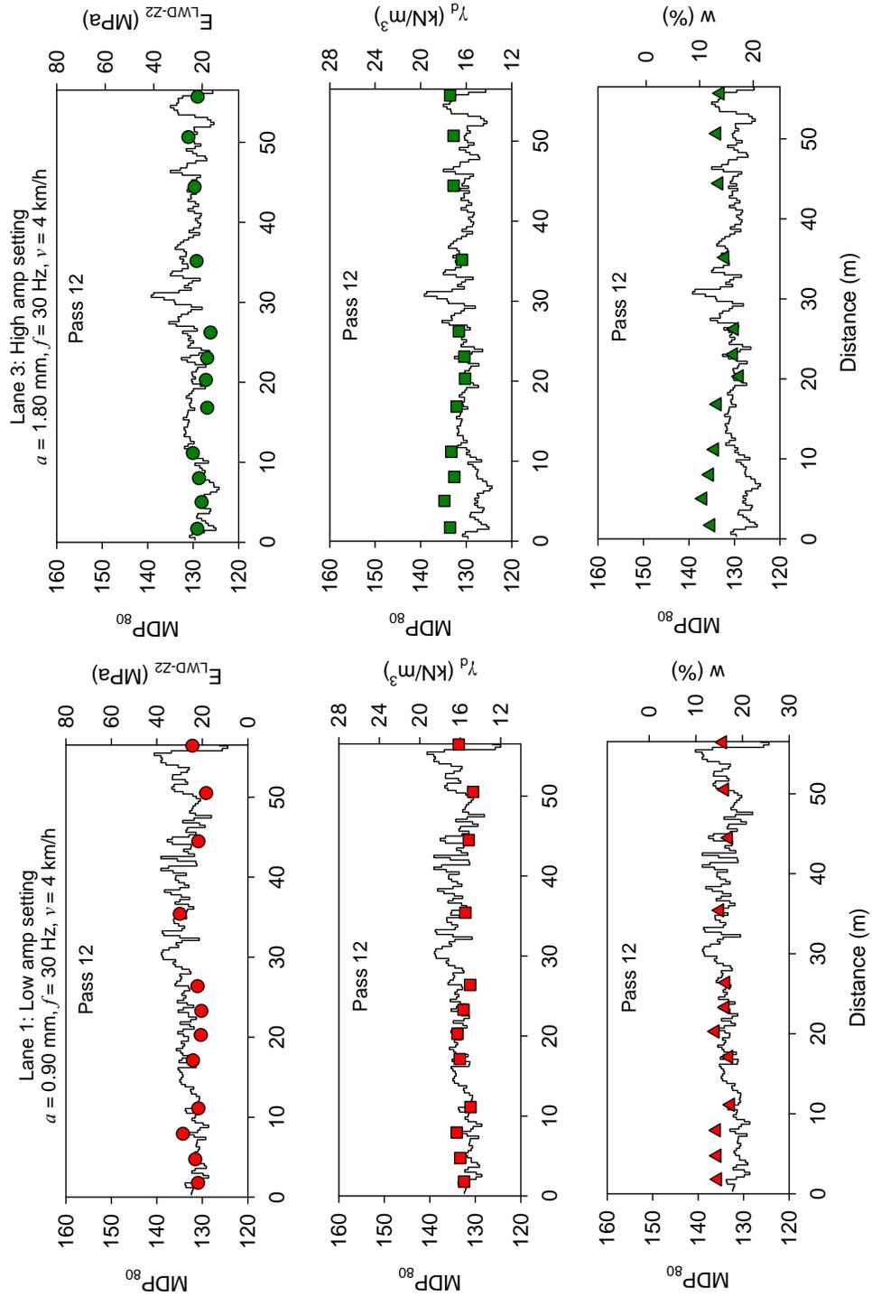
**Figure 19. Comparison between pass 12  $MDP_{80}$  measurements and in-situ point measurements on TB2 lanes 1 and 3 subgrade clay material**
