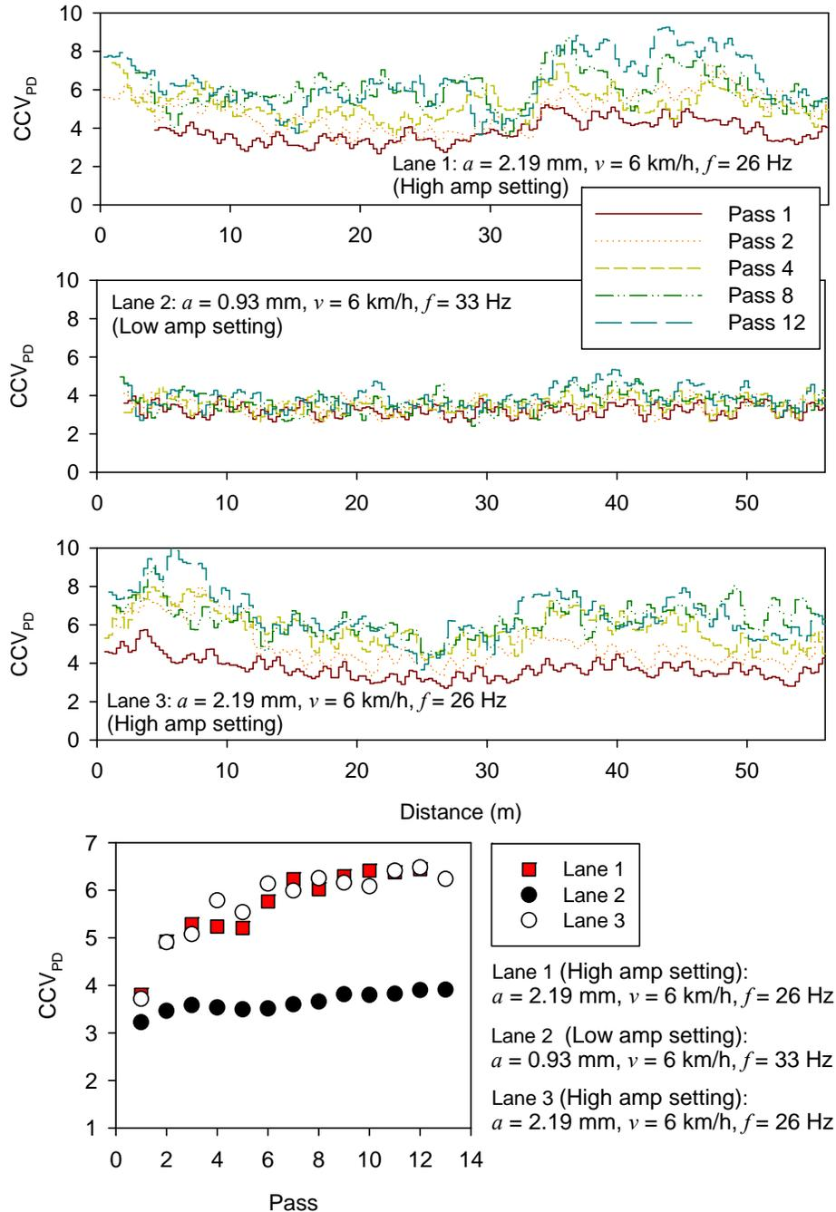
**Figure 26.  $CCV_{PD}$  measurements for multiple passes and compaction growth curves on TB4 subgrade clay material lanes 1, 2, and 3**
