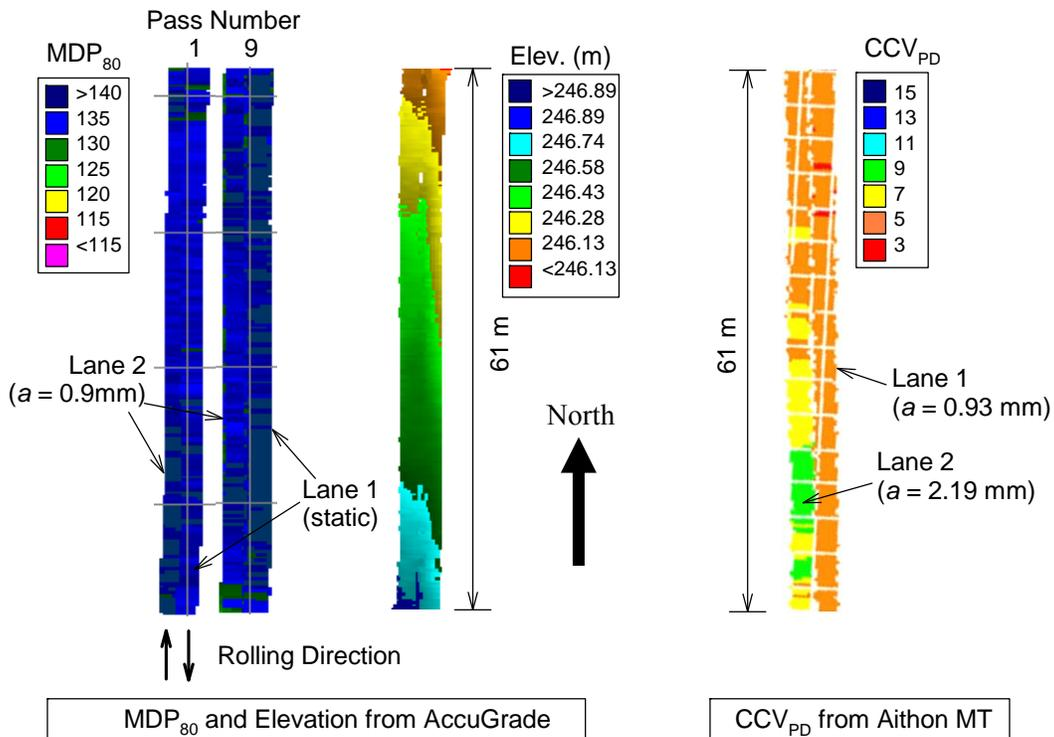
Figure 7. MDP<sub>80</sub> and elevation maps from Caterpillar AccuGrade software and CCV<sub>PD</sub> map from Sakai Aithon MT software – TB1 subgrade clay material lanes 1 and 2
