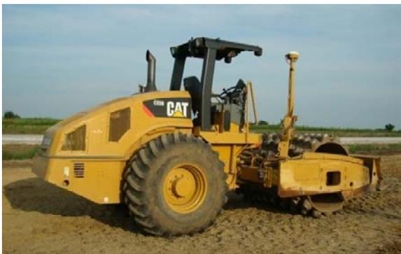
*Caterpillar CS56 padfoot roller used for compaction*
