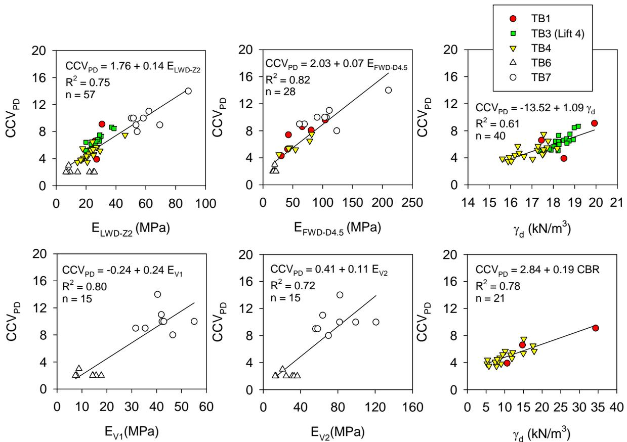
**Figure 55. Regression relationships between  $CCV_{PD}$  and in-situ point measurement values from TBs 1, 2, 3, and 4 calibration test strips, and TBs 6 and 7 ( $a = 2.19$  mm,  $f = 26$  Hz)**
