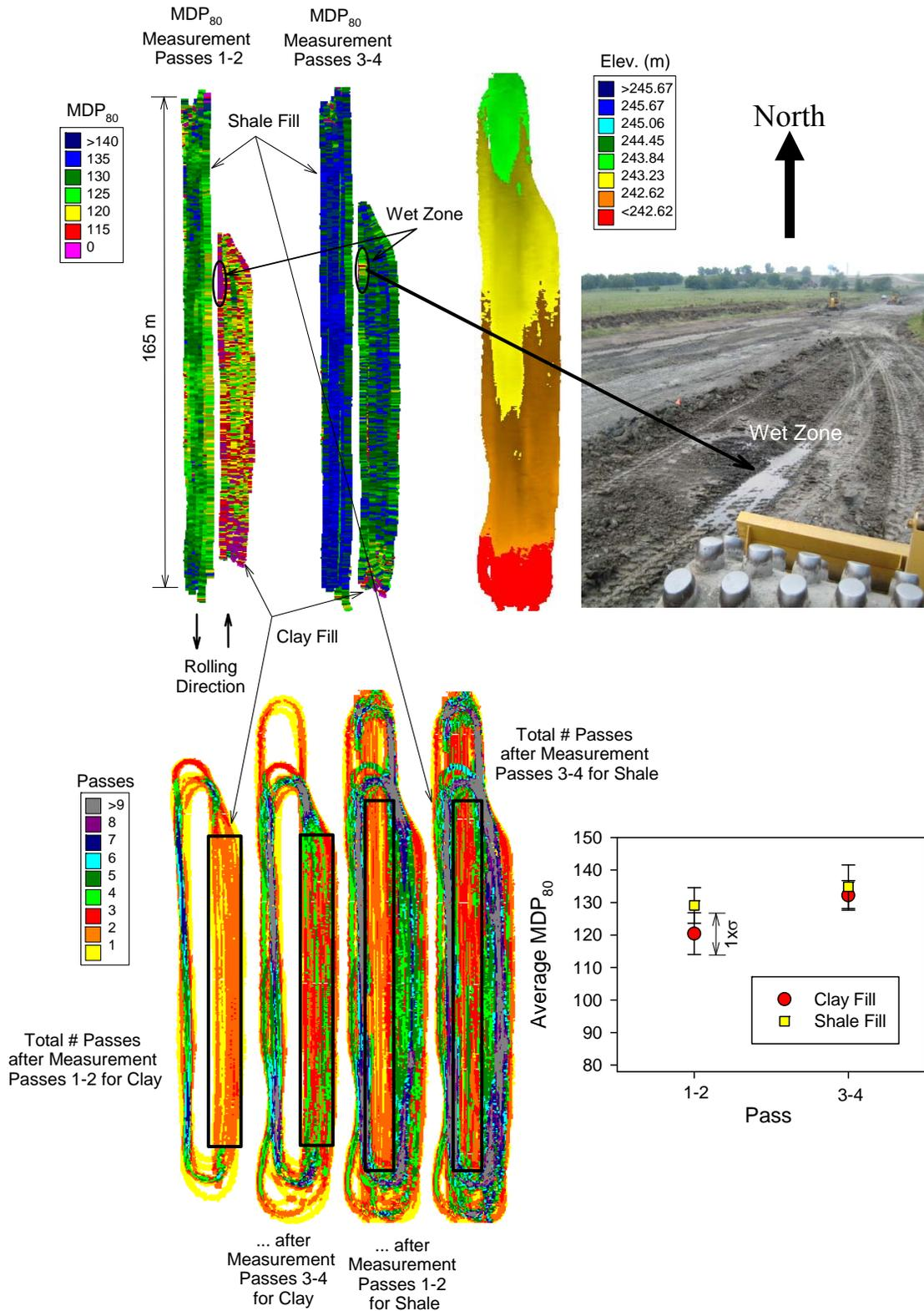
**Figure 37. MDP<sub>80</sub>, elevation, pass coverage, and average MDP<sub>80</sub> ( $a = 0.90$  mm,  $f = 33$  Hz,  $v = 4$  km/h) per pass on TB3 lift 1 clay fill and shale fill material**
