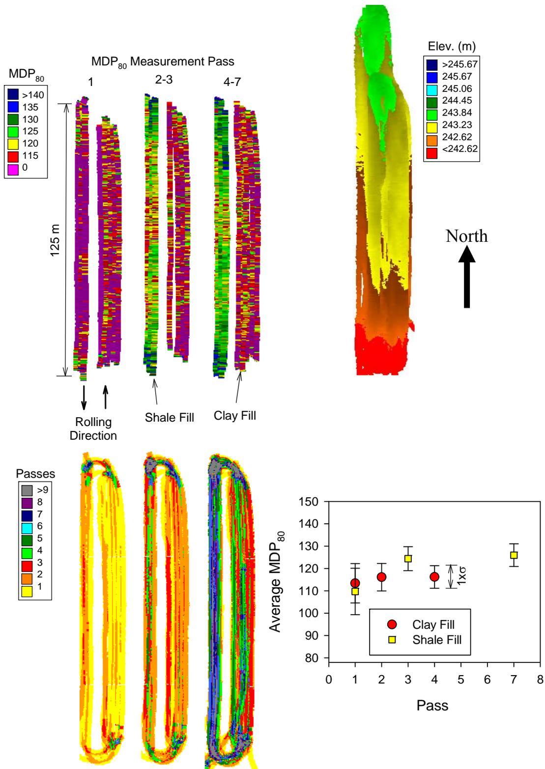
Figure 38. MDP<sub>80</sub>, elevation, pass coverage, and average MDP<sub>80</sub> ( $a = 0.90$  mm,  $f = 33$  Hz,  $v = 4$  km/h) per pass on TB3 lift 2 clay fill and shale fill material
