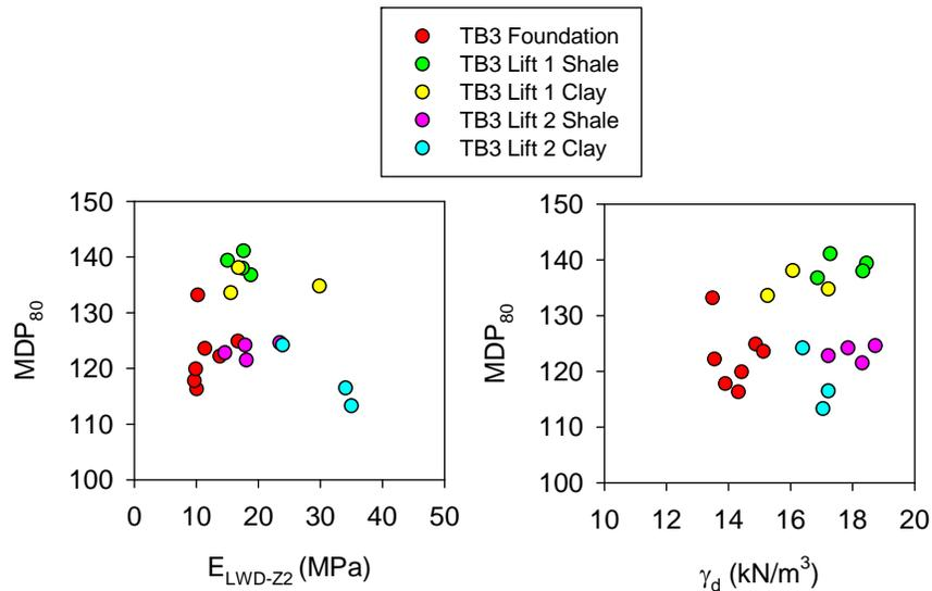
**Figure 63. Regression relationships between  $MDP_{80}$  ( $a = 0.90$  mm,  $f = 33$  Hz) and in-situ point measurement values – TB3 foundation layer and lifts 1 to 2**
