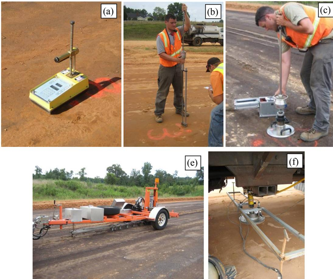
Figure 8. In-situ testing methods used on the project: (a) Humboldt nuclear gauge, (b) dynamic cone penetrometer, (c) Zorn light weight deflectometer, (d) Dynatest falling weight deflectometer, (e) static plate load test
