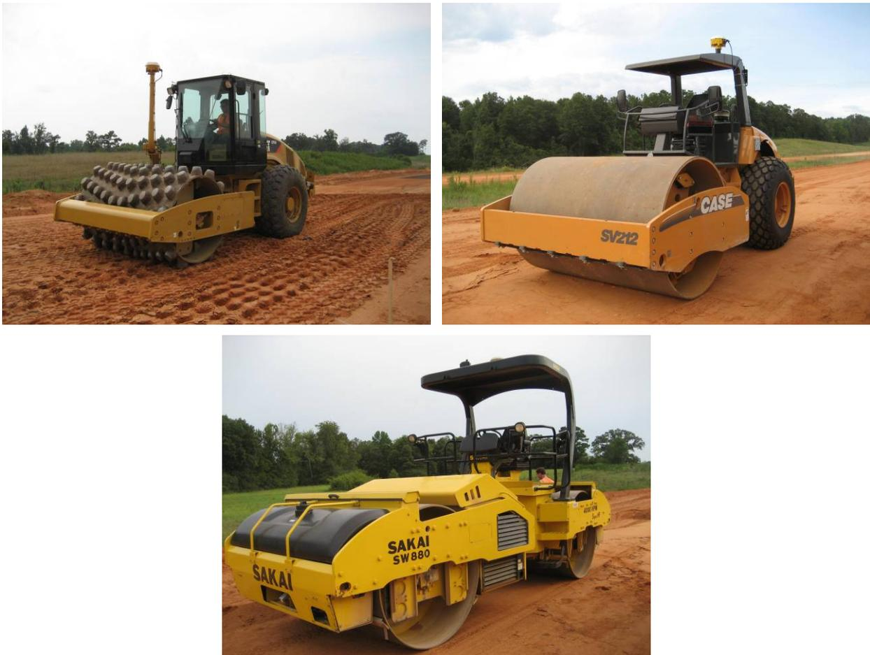
**Figure 1. Caterpillar CP56 (top left) padfoot, Case SV212 smooth drum, and Sakai SW880 dual smooth drum IC rollers used on the project**
