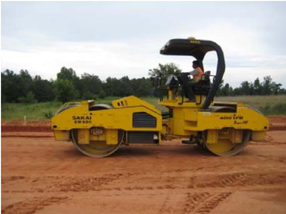
*Sakai SW880 roller used on the test bed*
