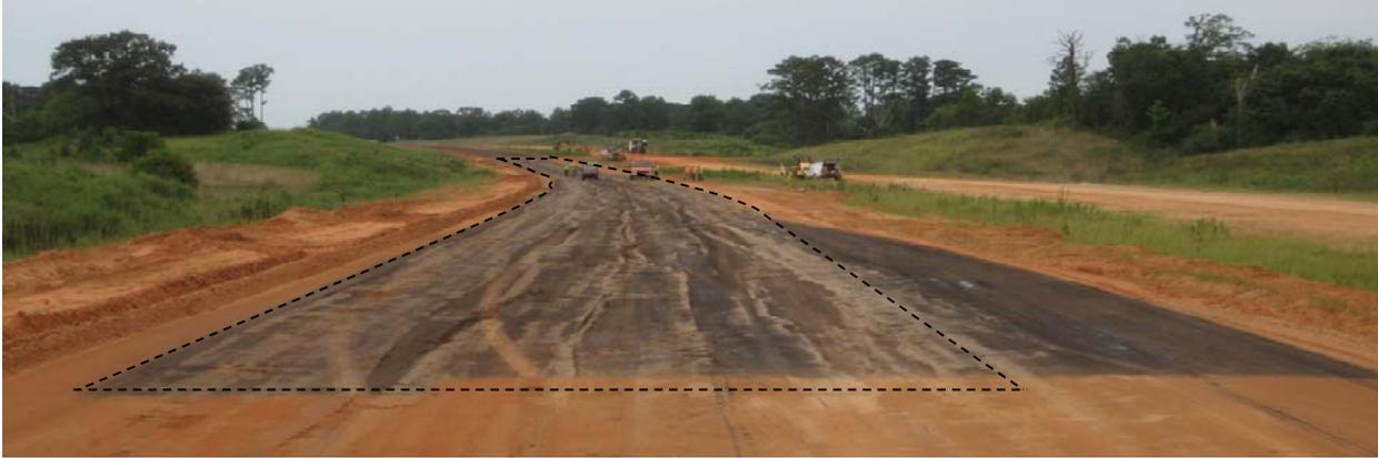
**Figure 14. Picture of the test bed – TB2 treated base material**
