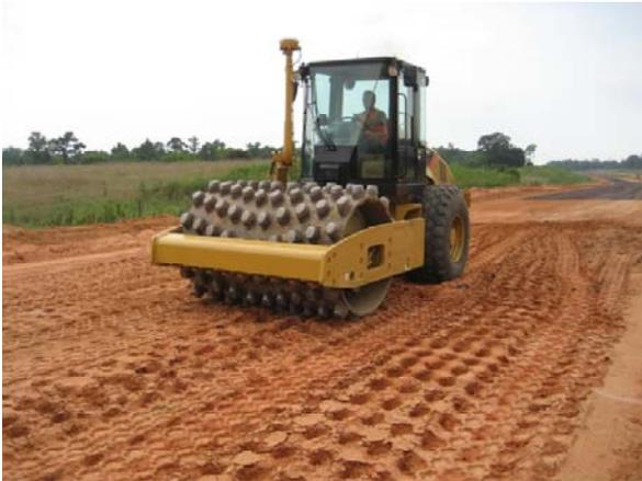
*Caterpillar CP-56 roller used on the test bed*
