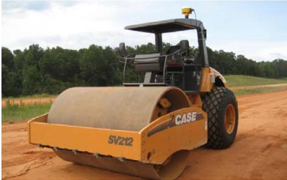
Case/Ammann roller used for mapping
